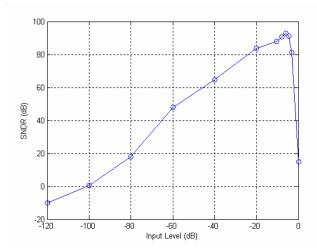
Figure 9. The dynamic range of the modulator
