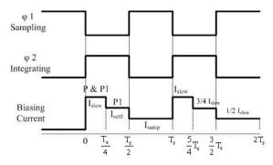
Figure 7. The clock phases of dynamic biasing circuit.
