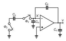
Figure 3. The SC integrator during the slewing and settling phases (φ2).
