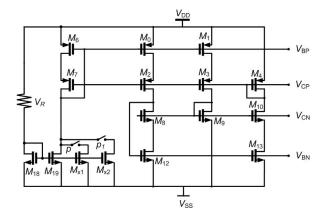
Figure 6. The dynamic biasing circuit.
